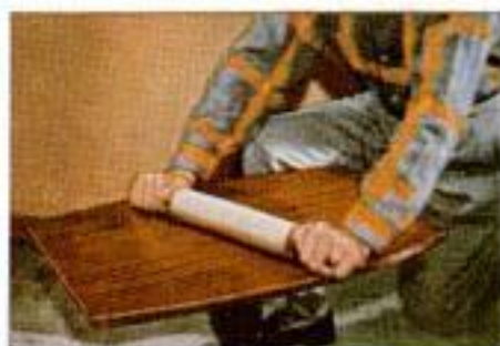
6. Roll with ordinary rolling pin and file edges.
